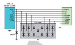
The maximum data rate in SuperSpeed mode is 5 Gbit/sec. The combination of USB 2.0 functionality and the new SuperSpeed mode requires a new cable construction. This is to accommodate serving three differential coupled signal lines (TX+/Tx-, RX+/Rx and D+/D-). The VCC and the GND line complete the cable set.
